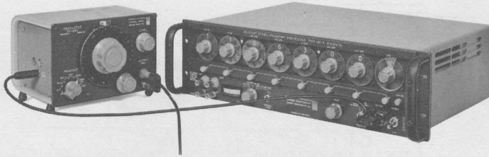
Figure 4-3. The Type 1309 Oscillator being synchronized with the Type 1161-A7C Coherent Decade Frequency Synthesizer.
